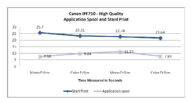
Application Spool Time and Time to Print was measured using both Color and Mono modes. The files were printed on 'E' and 'D' paper sizes using High Quality on Satin Photographic Paper.
