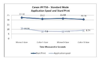
Application Spool Time and Time to Print was measured using both Color and Mono modes. The files were printed on E and D paper sizes using Standard Mode on Plain Paper.
