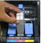
Removing the ink tank is easy. After lifting up the cover, the user pulls up on the tank cover (left), then grasps the tank and carefully pulls up and out (right).
