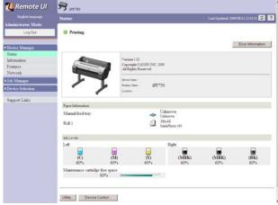
Users, key operators, and network administrators can check printer status through the Remote User Interface by typing in the IP address of the printer.
