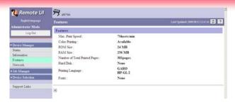
The Remote UI features tab, allows users to access features such as the total number of pages printed, speed, memory and hard disk information.
