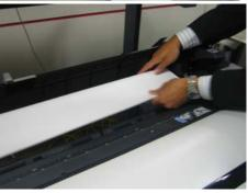
Above Clockwise: In order to change the paper roll, the user lifts out the paper roll from behind the print housing, then removes the roll holders from one end of the roller, slides out the old media roll, slides on the new media roll, then replaces the roll holder and tightens the clamp, replaces the paper roll and closes the roll cover.
