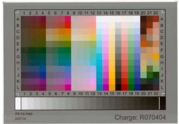
The scanned IT8 test chart
