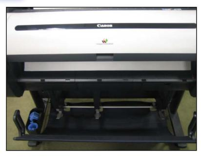
The iPF750 can be configured so that printed output automatically rolls around this bottom spindle. An optional basket can also be installed for catching prints. To remove the printed output, the user removes the spindle and one collar, and then slides it off the roll.
