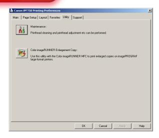
The Utility tab is for maintenance operations and launches the Status Monitor Maintenance tab (see Status Monitor).
