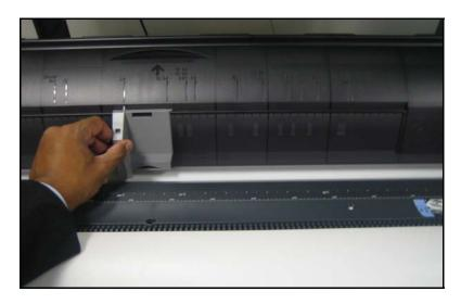
Easy cut sheet loading with built-in media guide
