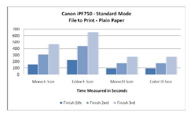
Side by side view of the mono and color files printed by paper size using Standard quality and plain paper.
