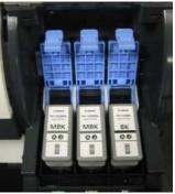
The imagePROGRAF iPF750 utilizes 5 color inks. The three colored (C, M, and Y) ink tanks are housed on the top left side of the printer, and three black (B and MBKx2) ink tanks are located on the top right side.
