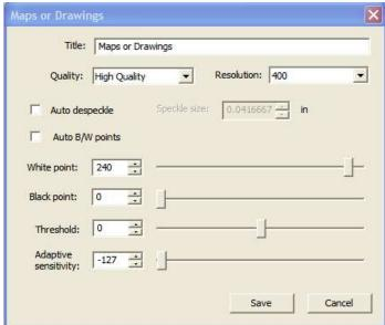
Black and white scanning has Adaptive thresholding for cleaning up faded or deteriorated drawings. This feature is often missing on black and white MFP systems.
