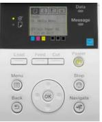
After installing new media, the LCD panel on the iPF750 prompts the user to specify the newly installed paper type. You should note that the iPF750 printer automatically detects media width.
