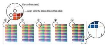
The Graphtec SK280 scanner color calibration sheet.
