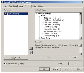
The Favorite tab is a nice addition where the user can save printer settings and recall them later. This feature was called Profiles in previous driver versions. With the ever-increasing list of options and parameters that can be specified to a printer, the need to recall previous settings provides users with great ease. BERTL really likes this feature because it makes life easier for the users.
