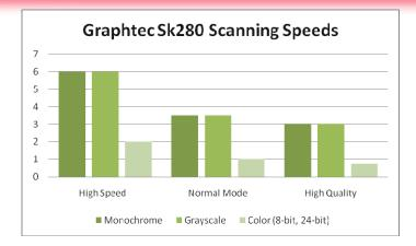
Scanner performance is in the mid-range, with a rated color speed of 2 ips at 400 dpi and black and white speed of 6 ips at 200 dpi, when using High Speed mode. One of the first things BERTL noticed is that, contrary to Graphtec's other scanners, the CIS sensors are located in the top lid of the scanner, so document loading is done face up. This is better than placing documents face down where you can't see the image you are loading.
