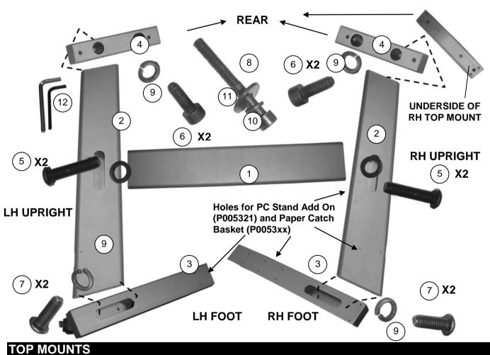
Attach scanner top mounts (item 4) to leg uprights (item 2) using 4 x socket head bolt (item 6) and 4 x split washer (item 9). Ensure the elongated hole of each top mount faces to rear of stand (shown) and the one with four small holes on the underside is fitted to the RH leg upright. This facilitates attachment of the optional Keyboard and Monitor Add-On kit.
